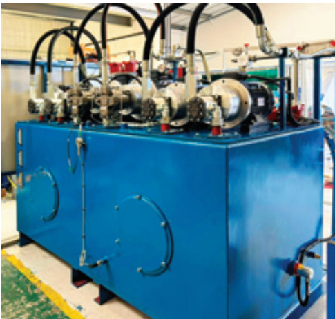
◀ Hydraulic unit undergoing factory acceptance test
