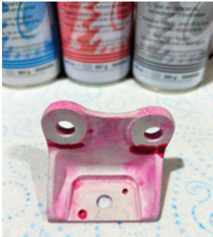
Retraining at Salvtech in dye penetrant testing has strengthened the company's culture of precision, safety and continuous improvement
