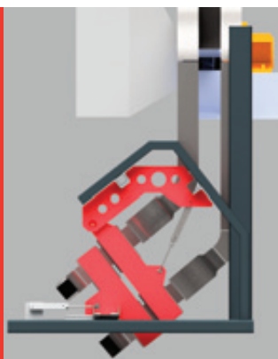
▶▶ Compact's Apollo dryer with reflector frames closed in the operating position (left) and open for maintenance (right)
