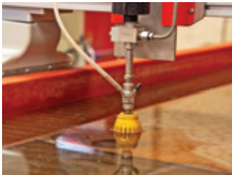
Latest water jet cutting equipment at T&S achieves precision cutting of 2D profiles up to 75mm thick
