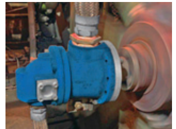
The new H68-Series of rotary pressure joints from Deublin directly replace the H67 units
